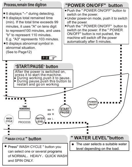
Remarks: After pressing "Power On/Off" to connect power supply, if the washing machine lasts idle more than 5 min, it would automatically shut off the supply.
